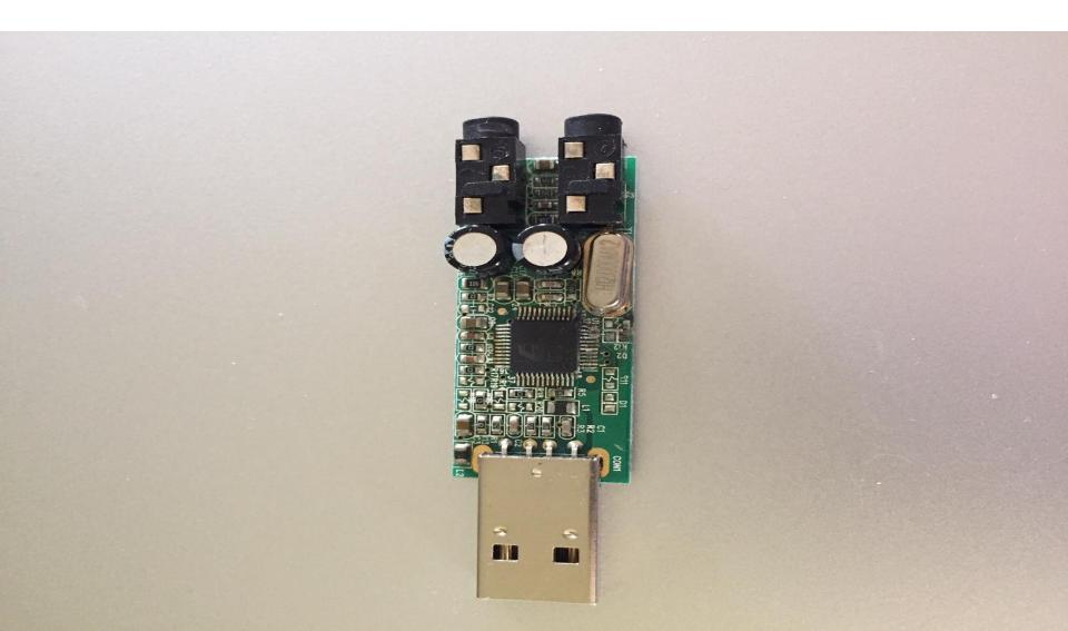
I chose to remove the audio jacks, to many problems with the 3.5mm plugs/jacks. This opens up the board and allows for easier removal of the mic bias resistor R122. This chip resistor (R122 - 1.2k ohm) normally supplies voltage to the microphone. This removes the voltage on the receiver discriminator audio input to the sound card eliminating the need for another coupling capacitor. Remove R122.
