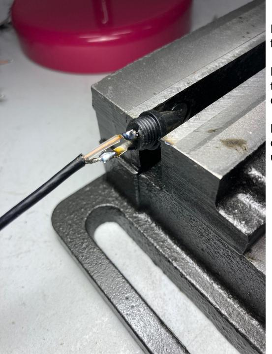
PTT RCA female straight connection from the 2n2222 collector pin.
