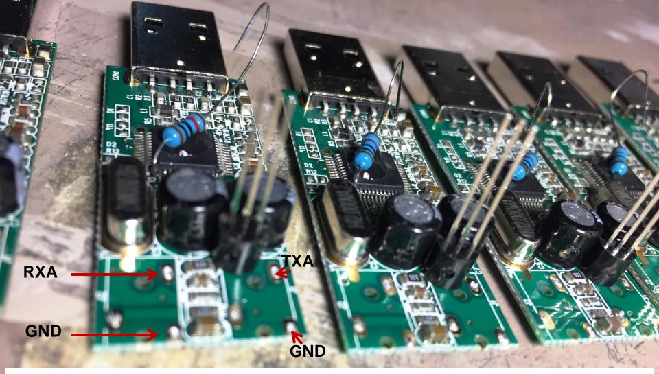
3.5mm jacks removed. 10k soldered to pin 13 of cm108 chip, then hot glued to cm108 chip, 10k will connect to base of 2n2222 for PTT.
