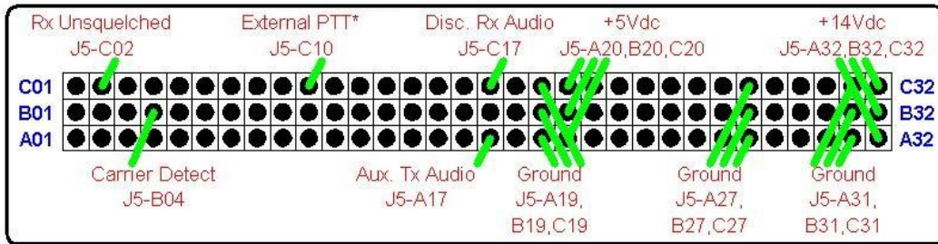
This image is looking at the 96-pin connector from the rear of the repeater. Again, we will not use all these connections. This image is for reference only.
